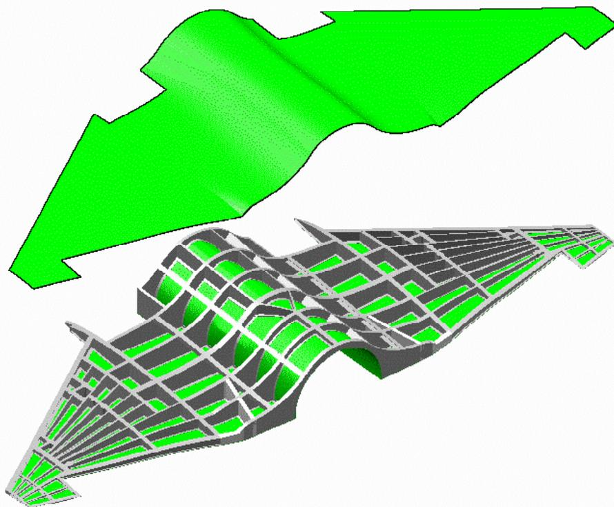
Figure 5. Upper tip-to-tip wing carry through skin panel with mating frame assembly (understructure) shown below.
