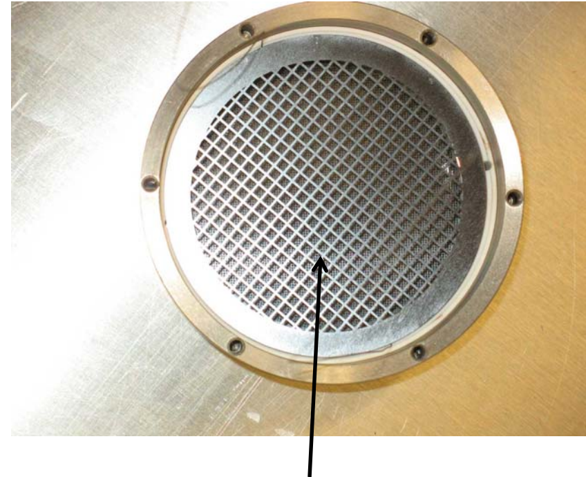
Faraday Cup with SiC grid in place
